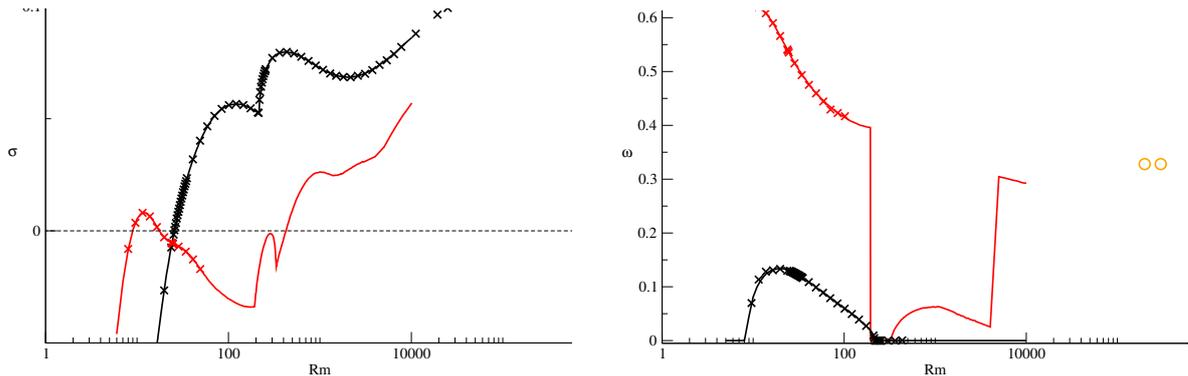
Fig. 4: Real (left) and imaginary (right) part of the leading eigenvalue associated to the V symmetry family (black) and the II symmetry family (red), in the classification introduced by [JG14]. Continuous lines correspond to the results published in [JG14]. Crosses present our numerical results in [BD13] and in the present study. Circles denote the transient behaviour.
