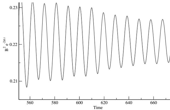
Fig. 3: Damped oscillations in the time evolution of the magnetic energy corrected for the averaged exponential growth rate at  $Rm = 2 \cdot 10^5$ .
